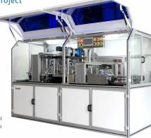
Fully automated material feeding,automat ed sensor mark positioning, automated pu nching, automated skeleton off-take.
